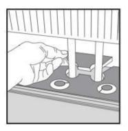
Installation at radiators. Drill the holes 20 mm larger than the diameter of the pipes.
